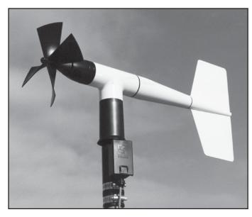
The **Model 200-05103 Wind Monitor** is a high performance, rugged wind sensor. Its simplicity and corrosion-resistant construction make it ideal for a wide range of wind measuring applications. The instrument is made of UV stabilized plastic with stainless steel and anodized aluminum fittings. Precision grade, stainless steel ball bearings are used. Transient protection and cable terminations are in a convenient junction box. The instrument mounts on standard 1" pipe.
