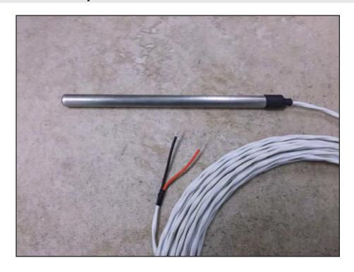
The **210-101W Water Temperature Sensor** is a rugged and reliable device for highly accurate submersible water temperature or soil temperature measurement. It produces a 4-20 mA output signal, which is an industrial standard for process control monitoring. Most PLCs (Programmable Logic Controllers), SCADA equipment, and data acquisition systems accept this signal directly.
