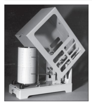
The **Model 225-5020-A Hygrothermograph** is a precision, self-contained instrument that measures and records ambient temperature and relative humidity simultaneously on a double scale chart. It is ideal for measurements in laboratories, computer rooms, libraries, museums, or agricultural areas.
