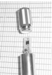
reapplying power to the probe. Replace the membrane filter if it appears to be frayed or cut. The filter may be cleaned with a soft bristle brush to remove any loose dust or dirt.
