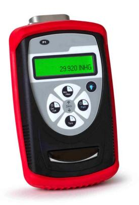
The Precision Absolute Manometer is a microprocessor based pressure sensing device used to directly measure pressure relative to absolute zero. Pressure can be displayed in a variety of engineering units. All units include a Tare function, a Min/Max function, selectable damp rates and altitude displayed in feet or meters. The manometer can also display barometric pressure corrected to sea level.
