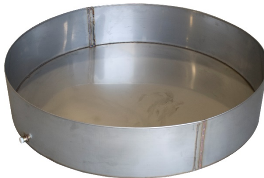
FIGURE 4-2. 255-200 Novalynx Class A Evaporation Pan
