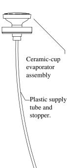
(3) Now load this assembly onto the water reservoir tube. The gray plastic part is secured to the top of the reservoir by two spring clips. Before snapping the top assembly down, fill the reservoir to the zero mark on the scale. (See a later page of these
