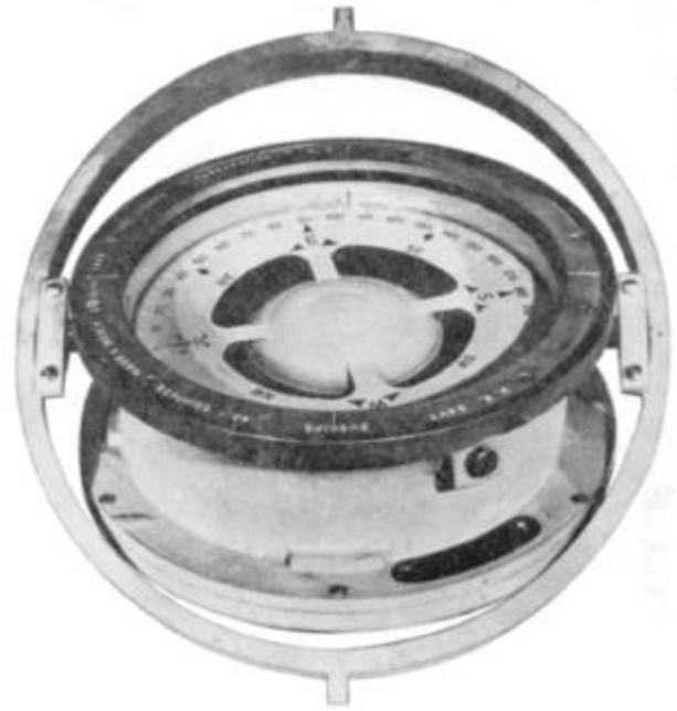
Figure 2-28—Shipboard magnetic compass.
