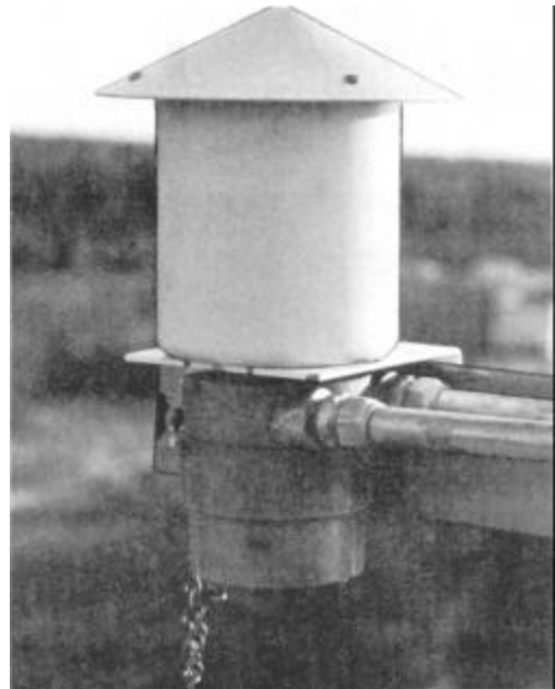
Figure 2-11.—ML-643/GMQ-29 dew-point sensor.
