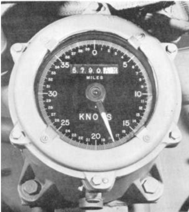
Figure 2-30.—Shipboard underwater-speed log indicator.
