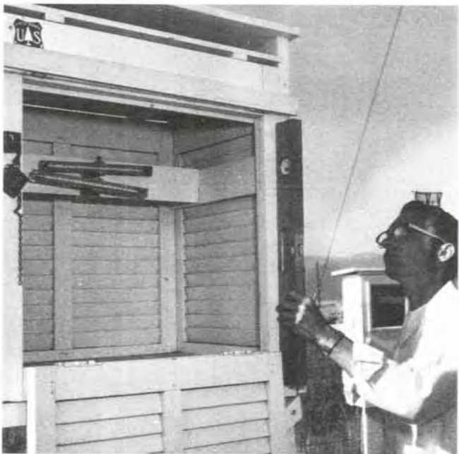
Figure 16.2—Installing and leveling instrument shelter using mounting pins.
