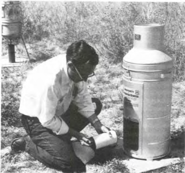
Figure 25.1—Operating procedure for Universal weighing gauge: A, remove the collector, after releasing pen from chart; B, empty bucket; C, remove chart drum and install new chart; D, wind clock; E, replace chart drum and zero the pen.
