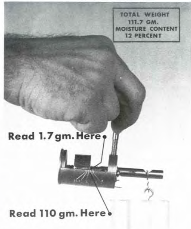
Figure 26.7—Weighing the fuel stick on Williams pocket scale. The stick weighs 111.7 grams, so its moisture content is 12 percent as indicated on scale.
