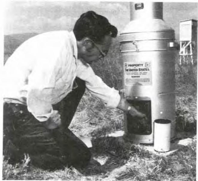
Figure 25.1—Operating procedure for Universal weighing gauge: A, remove the collector, after releasing pen from chart; B, empty bucket; C, remove chart drum and install new chart; D, wind clock; E, replace chart drum and zero the pen.
