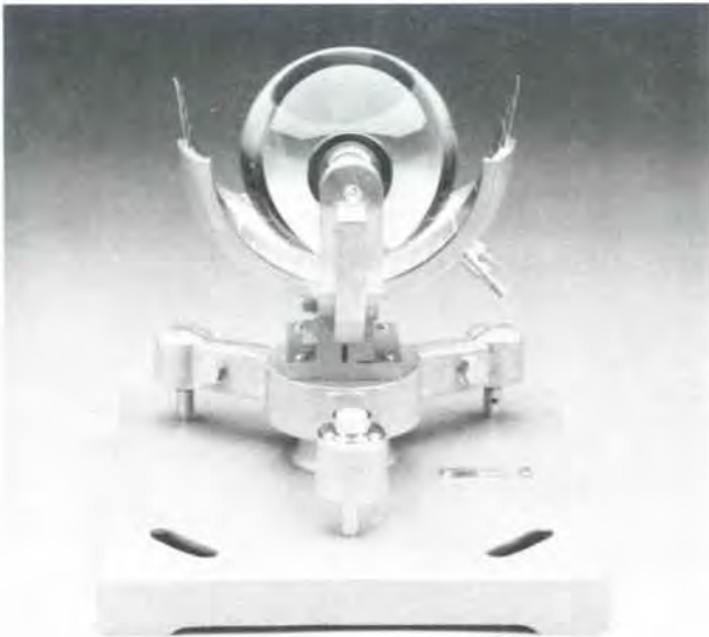
Figure 11.1 —Campbell-Stokes sunshine recorder. (Photo courtesy of Qualimetrics, Inc.)
