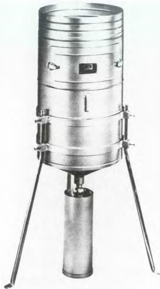
Figure 9.9—Tipping bucket rain gauge containing reservoir, with tube for stick measurements; standard NWS design with 12-inch-diameter orifice. (Photo courtesy of Belfort Instrument Company.)
