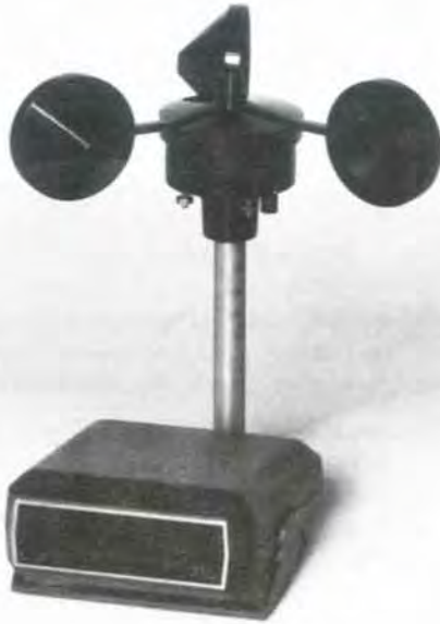
Figure 8.10 —Accumulating-type generator anemometer, Natural Power model A19-S6A; digital readout gives 10-minute average windspeed. (Photo courtesy of Controlex, Inc.)
