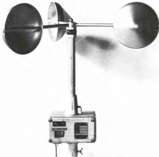
Figure 8.5 —Totalizing anemometers equipped with both \frac{1}{60} -mile and 1-mile contacts: top left, instrument with self-contained readout dial; top right, without self-contained readout; bottom, with self-contained readout counter.
