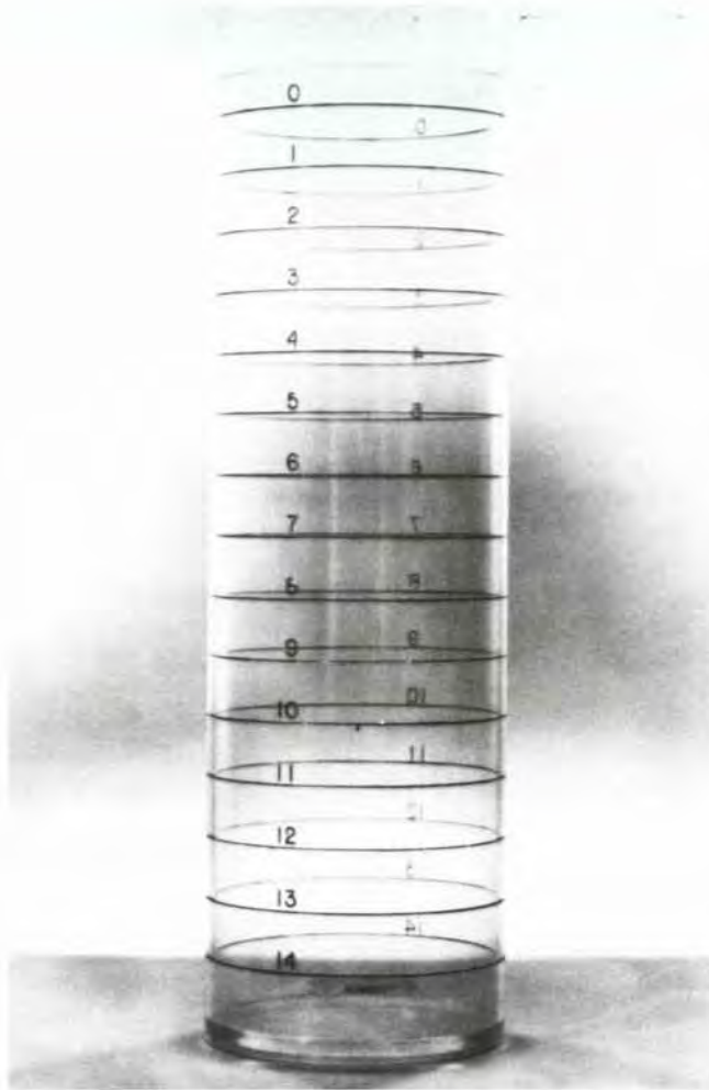
Figure 12.5—Plastic measuring tube used with fixed-point gauge. (Photo courtesy of Sierra-Misco, Inc.)
