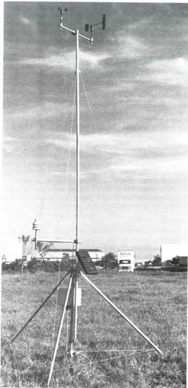
Figure 38.2—A portable RAWS, without satellite antenna. (Photo courtesy of Handar.)
