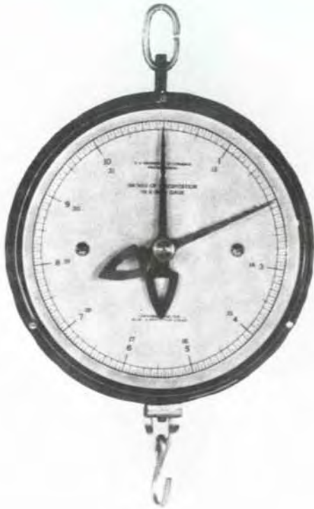
Figure 9.3 —Weighing scales, used with overflow can of large-capacity 8-inch rain gauge; a convenient means of measuring water content of snow. (Photo from U.S. Department of Commerce 1972.)
