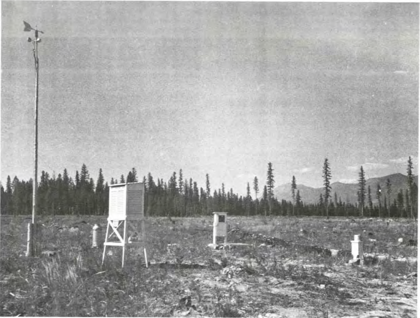
Figure 17.1—A standard anemometer installation 20 ft above open, level ground.
