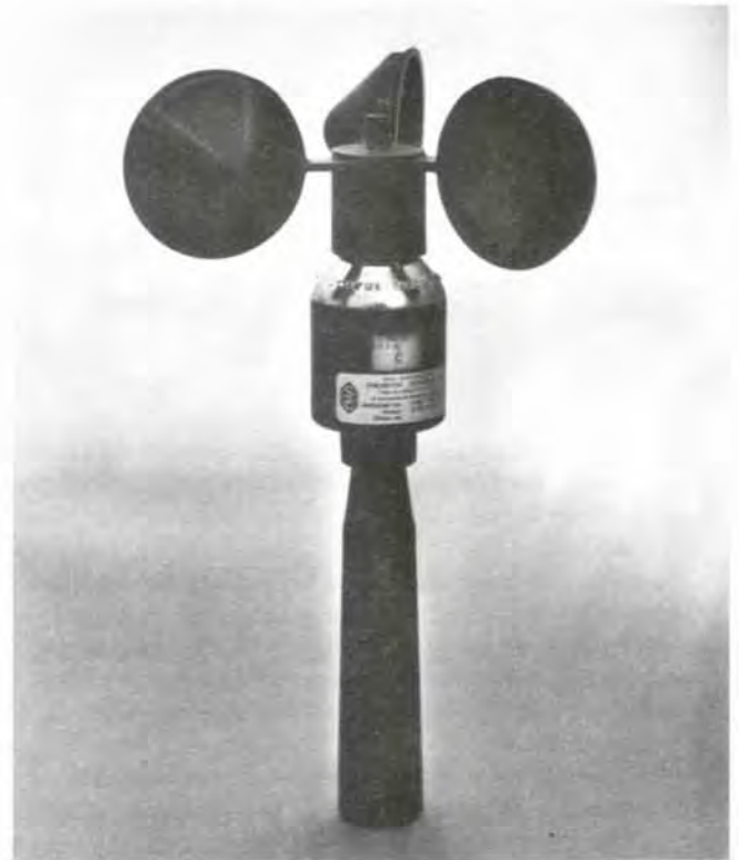
Figure 8.11 —Hand-held anemometer, with scale on rotating drum. (Photo courtesy of Qualimetrics, Inc.)
