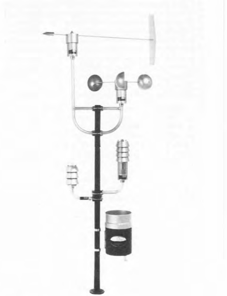
Figure 44.6 —Typical sensor array used in Texas Electronics (series 3000) modular meteorological system. (Photo courtesy of Texas Electronics, Inc.)
