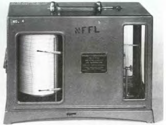
Figure 7.18 —Hygrothermograph, Bendix model, as normally exposed with case closed. The upper pen records temperature; the lower pen, relative humidity. Calibration adjustment screws are at right.
