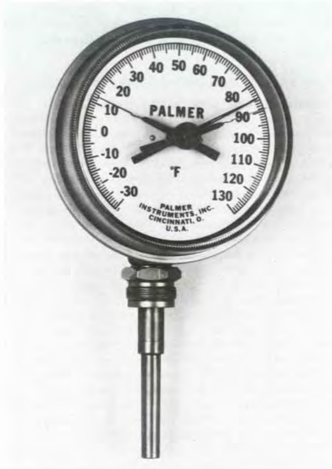
Figure 7.10 —Dial type maximum-minimum thermometer, employing a mercury-in-steel sensing element with direct-drive Bourdon spring. (Photo courtesy of Palmer Instruments, Inc.)
