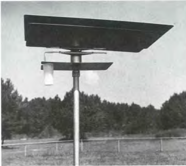
Figure 7.17 —The mortarboard psychrometer, with self-contained aluminum radiation shield; used in southeastern area of United States.
