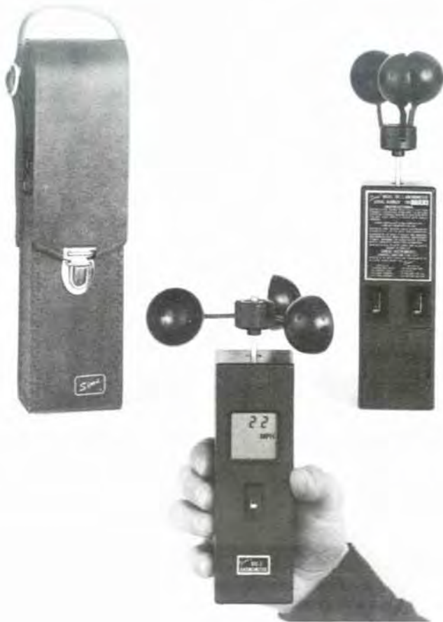
Figure 8.12—Hand-held anemometer with digital readout showing 2-minute or 5-minute average windspeed; Sims model DIC-3. (Photo courtesy of Simerl Instruments.)
