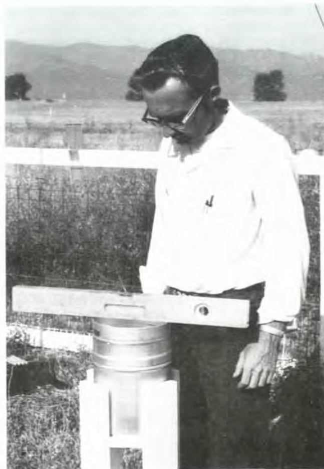
Figure 32.1—Checking the level exposure of a standard rain gauge (Forest Service type).
