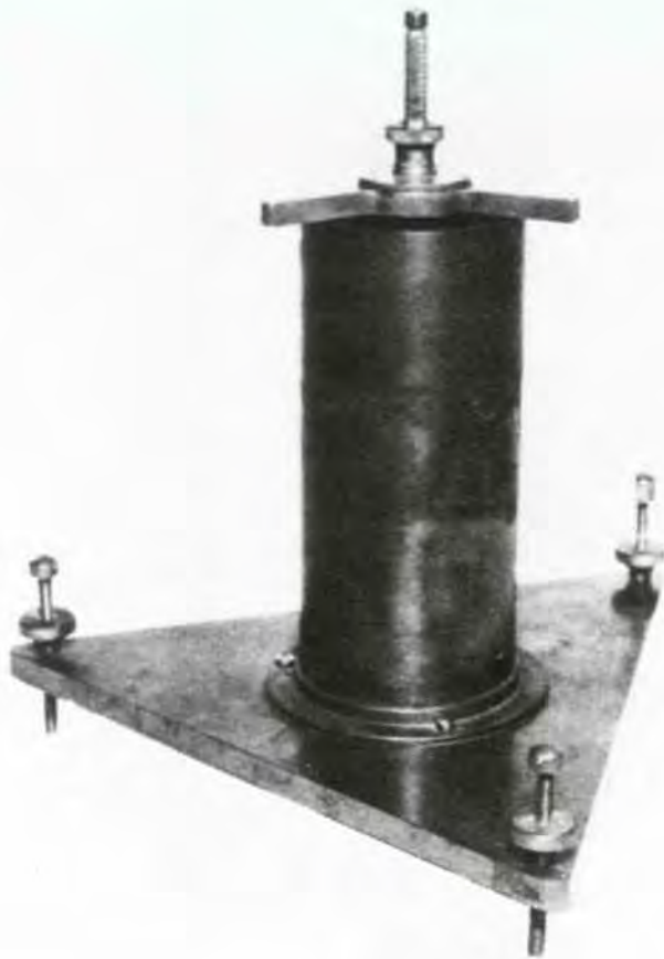
Figure 12.2 —Stilling well with hook gauge installed; leveling screws in base plate. (Photo from U.S. Department of Commerce 1972.)
