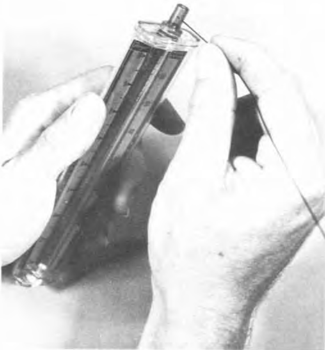
Figure 31.11—Top: cleaning, drying, and removing static from inner tube of Dwyer meter. Bottom: cleaning top stem pinhole.
