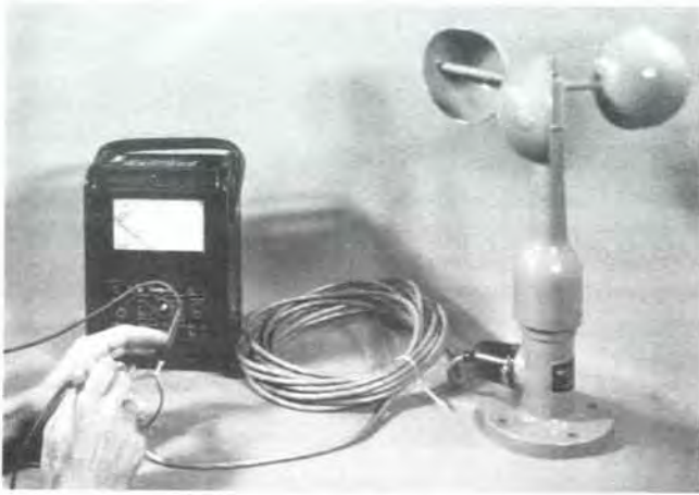
Figure 31.2—Using a continuity tester to check an anemometer circuit.
