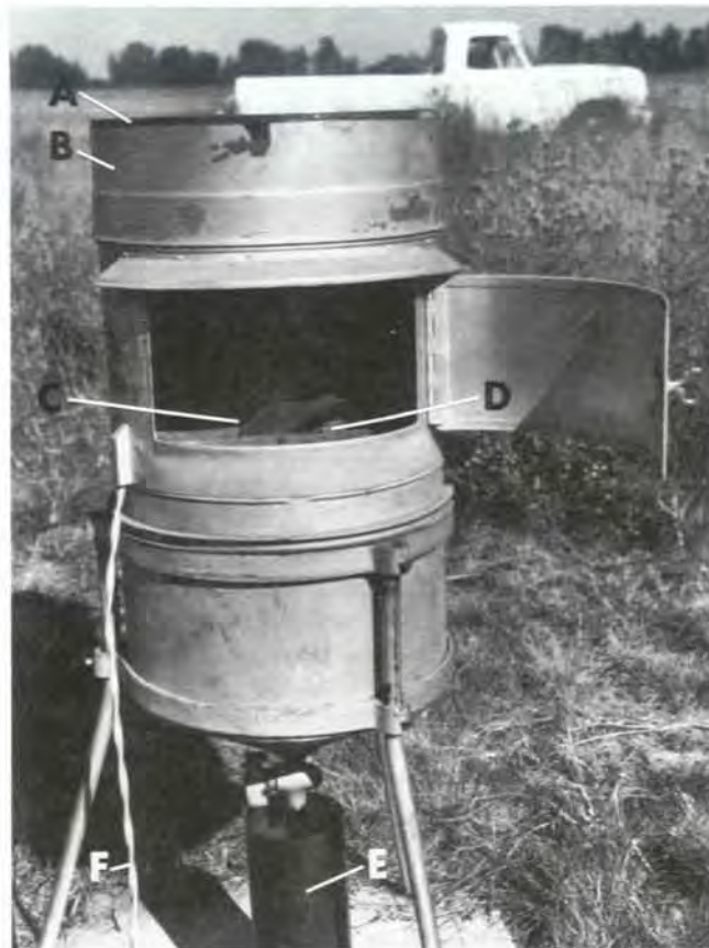
Figure 32.4—Tipping bucket precipitation gauge: A, collector rim ("knife edge"); B, collector; C, tipping bucket; D, calibration stop screw; E, measuring tube (for gauge with reservoir); F, cable to recorder.
