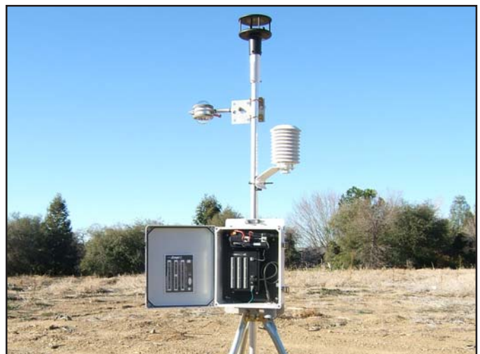
High Accuracy Ultrasonic Station
