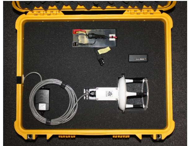
S10 Portable Weather Station with 200-91000 Ultrasonic Anemometer
