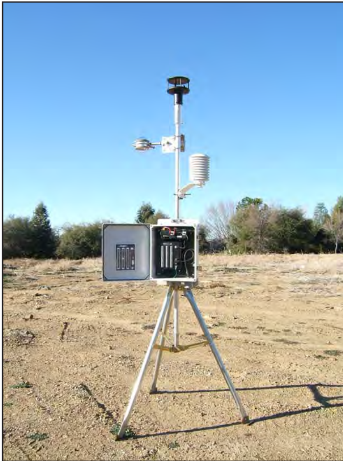
195-NL32N Data Logger (shown with weather station purchased separately)
