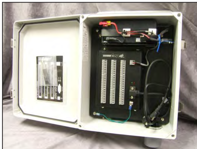
195-NL32 Data Logger in NEMA Enclosure
