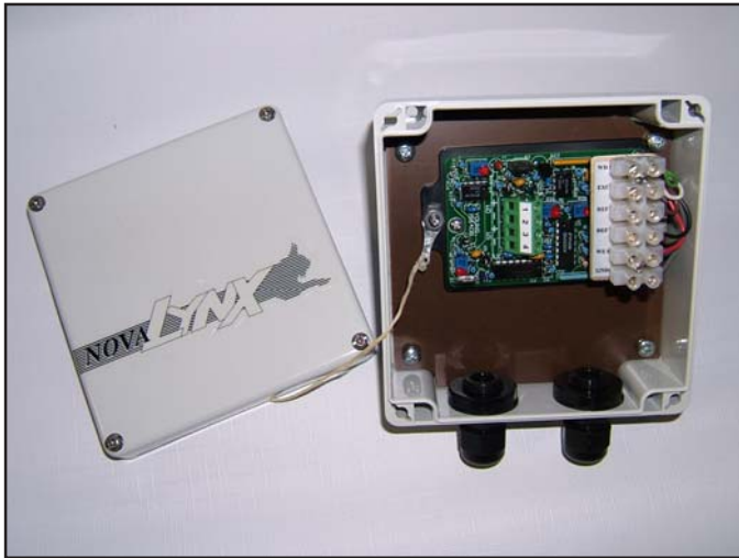
Current Loop Wind Sensor Printed Circuit Board in NEMA Enclosure
