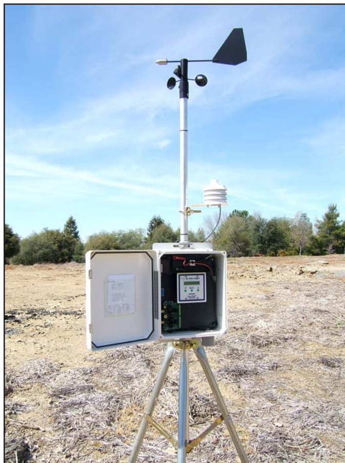
200-WS-25 Wind Logger with Real-Time Display shown with optional temperature sensor and shield, tripod, sensor mast, and mast mounting hardware
