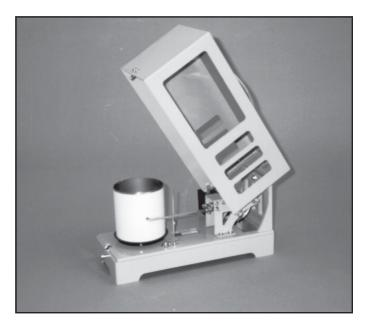
The **Model 210-4110-A Thermograph** is a precision, self-contained instrument that measures and records ambient temperature indoors or out. An aged bimetal strip expands and contracts with changing temperature. This movement is transferred to the pen through a counter balanced mechanical linkage. A span of 60°C or 110°F can be measured, and the span can be easily adjusted for different seasons.
