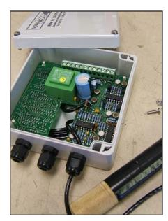
The **225-THT-1 Temperature & Humidity Sensor** is configured for measuring relative humidity and temperature in environmental control systems, where condensation or dust will commonly be encountered. A fully gasketed watertight enclosure, locking strain relief connections, and a brass sintered filter protect the electronics and sensors from environmental or mechanical damage.
