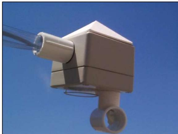
Both distance and air temperature are output as an analog signal between 0 to 2.5 Volts or 0 to 5 Volts. Measurements can be output digitally as serial ASCII. Specify analog or digital output at the time of order. Due to the simplified interface, the depth sensor can interface with any data logger or control system that can delay at least 3 seconds after powering up before measuring the output.
