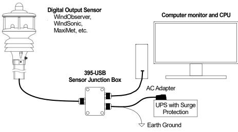
USB cable 5.9' (1.8 m), AC Adapter cable 3' (0.9 m), Earth grounding wire 5' (1.5 m), Sensor input cable (not included)
