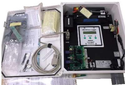
110-WS-25DL-N Data Logger with NEMA-4X enclosure (Interior: 10"w x 12"h x 5.27"d)
