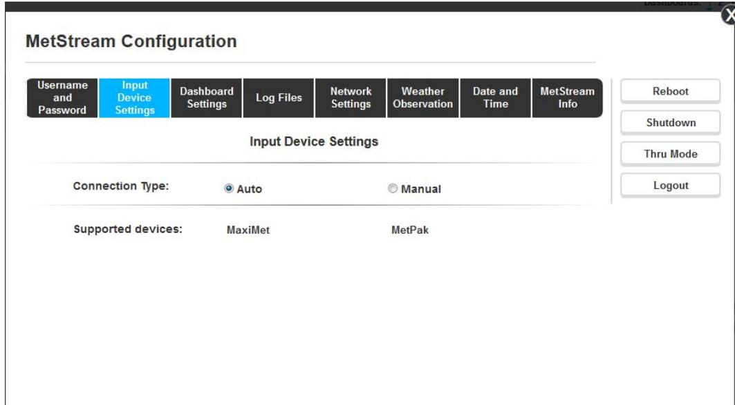
When Auto mode is selected then the connected device settings can be read and will be shown as per the following example with a connected MetPak Pro.
