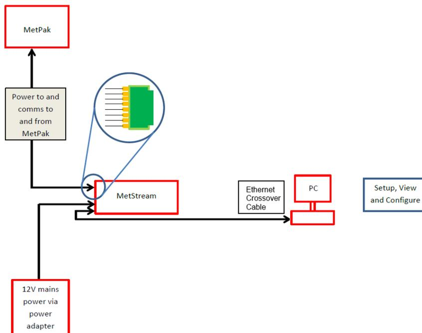
On first applying power to the MetStream 100, wait for 90 seconds before attempting to access it for data.
