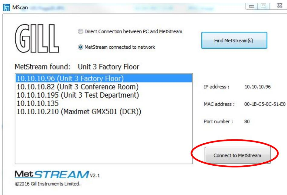
**NOTE the MetStream IP address is detected by the Wi Fi Router and can change each time MetStream is powered up if the MetStream unit is set for DHCP. Use Configure to fix the IP Address of MetStream if required.**
