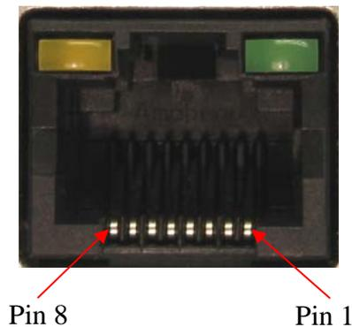
IEEE 802.3af connections using spare pairs for POE.
