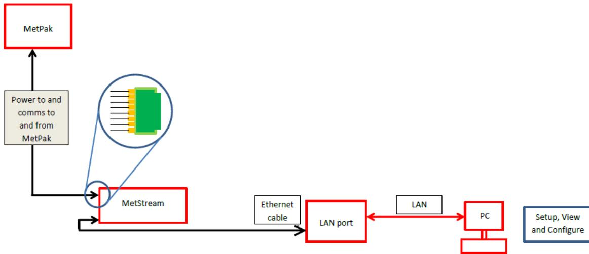
Connect MetStream to a LAN connection using the 2 metre Ethernet Cable supplied or any standard non crossover Ethernet cable.
