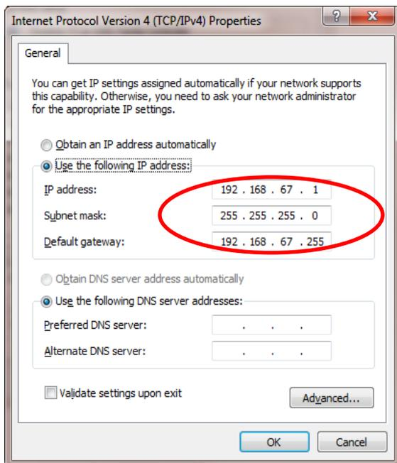
Type in the PC IP address **192.168.67.1** (cannot be the same as the MetStream default IP address 192.168.67.67).
