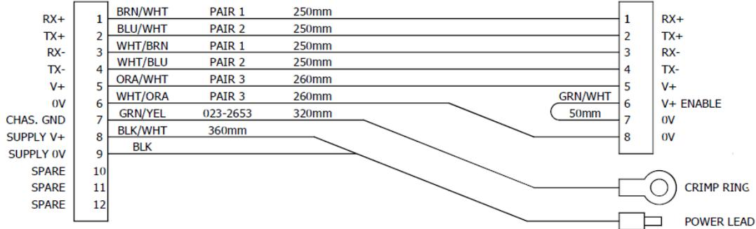
Connect external Power and Communications to the MetStream via the sealing strip or gland entry points and terminate in the 12 way screw fitting connector block.
