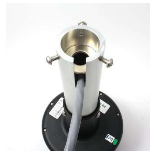
Bottom View showing large washer installed.
