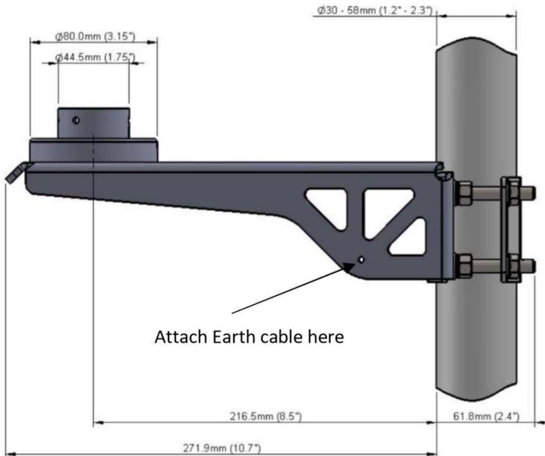
**\*Note:** Masts up to 76mm diameter can be accommodated provided longer bolts are used (not supplied). Fully threaded M8x100 mm recommended.
