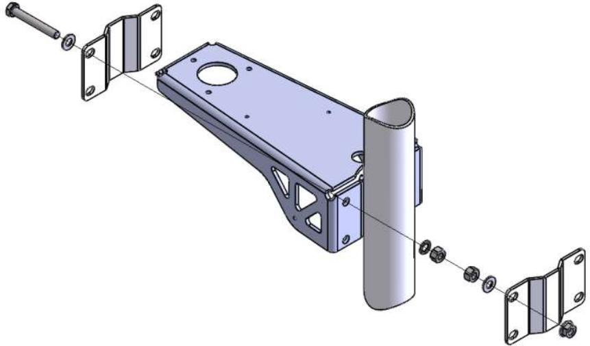
3. Hold the bracket to the mast and install the outer moving plate. For masts that are less than 1.5" diameter (38 mm) reverse the outer plate for a snug fit.
