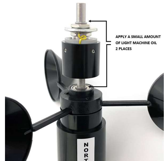
200-WS-02FA Sensor (vane assembly removed)
