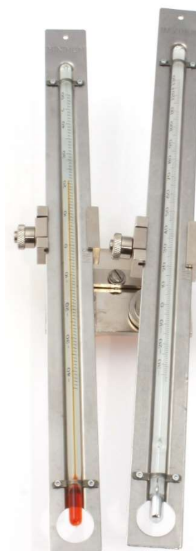
Minimum & Maximum Thermometers on Townsend Support
