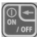
Turns the manometer on into the **Measure Mode** and then turns the unit off from the **Measure Mode**. Also serves as a backspace key ← when editing in the **Program Mode**. The backspace function takes the user out of a programmable register without changing the previous setting. Pressing this key repeatedly will return the user to the **Measure Mode** and then shut off the manometer.
