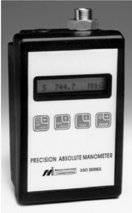
The Model 230-355 Precision Absolute Manometer is a microprocessor based pressure sensing device that can be used to directly measure absolute pressure. Models are available to measure pressure ranges up to 900mm HgA and 2000mm HgA. Pressure can be displayed in a variety of engineering units. All units include a Tare function, a Min/Max function, selectable damp rates and altitude displayed in feet or meters. The 355 can also display barometric pressure corrected to sea level.
