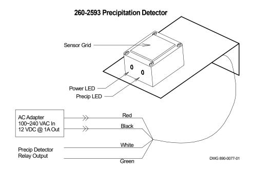
The internal relay is a dry-contact, normally open circuit. When connected to monitoring equipment, such as a logger, an open circuit represents no rain, and closed circuit indicates a rain event. The logger must supply a pull-up voltage to monitor the relay.
