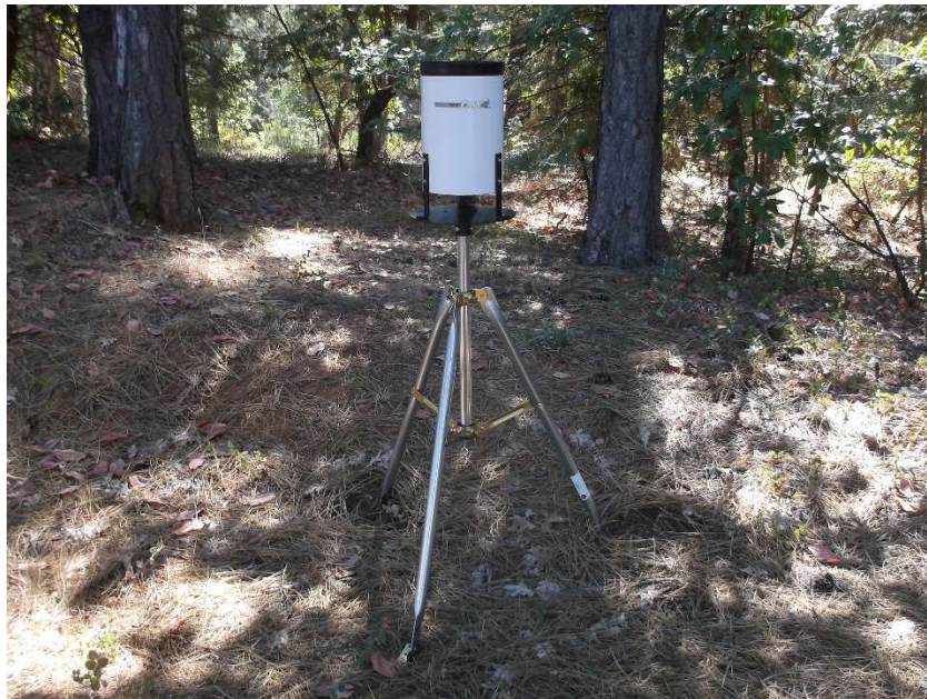
260-WS-2501 with Logger Mounted Inside the Rain Gauge
